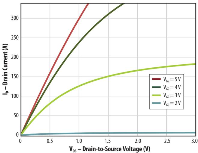
Figure 2: Transfer Characteristics
