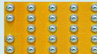
EPC2032 eGaN® FETs are supplied only in passivated die form with solder bumps. Die Size: 4.6 mm x 2.6 mm
