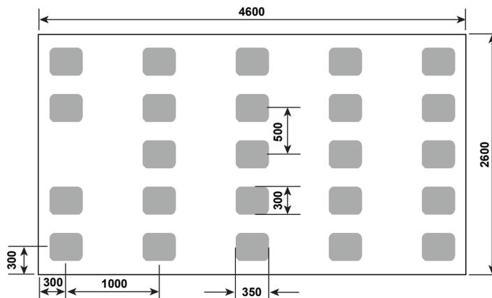
Recommended stencil should be 4mil (100  $\mu\text{m}$ ) thick, must be laser cut, openings per drawing.
