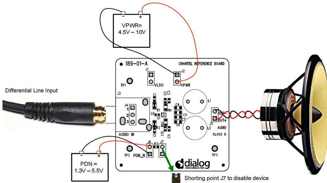
Figure 2: DA7202 performance EVB external connections
