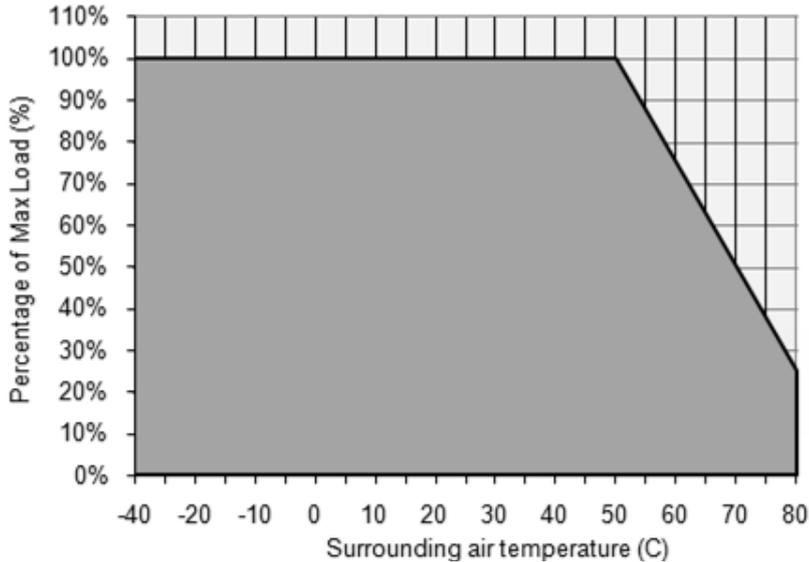
**Fig. 1 De-rating for Vertical and Horizontal Mounting Orientation**
