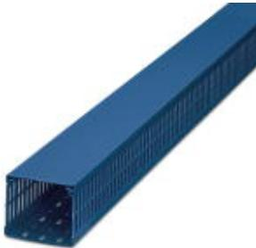
Wiring channel, blue, consisting of upper and lower part, width: 60 mm, height: 40 mm, length: 2000 mm
