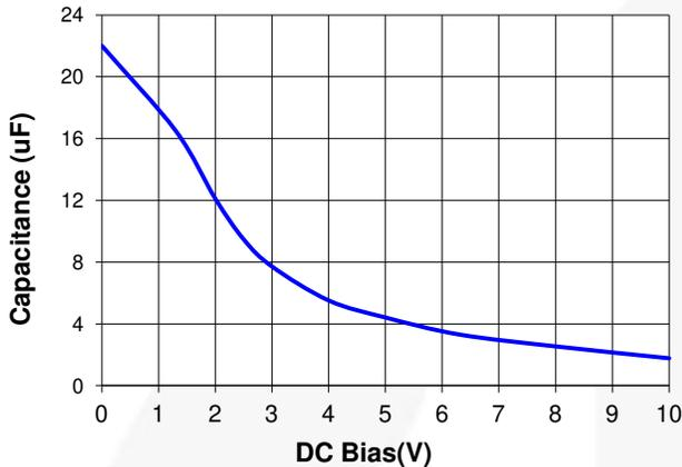
**Figure 40.** C<sub>EFF</sub> for 22 μF, 0603, X5R, 10 V-Rated Capacitor (TDK C1608X5R1A226M080AC)
