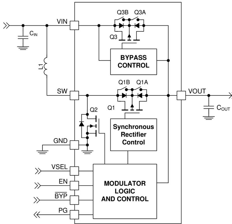
Figure 2. Block Diagram
