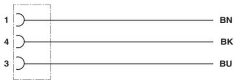
Contact assignment of M8 socket
