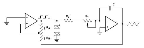
$\begin{array}{l} \mbox{frequency} \propto {\rm R_1, \, R_2, \, C} \\ \mbox{amplitude} \propto {\rm R_A, \, R_B} \end{array}$
