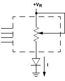
Two-terminal Variable Resistor; Variable current
