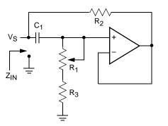
$Z_{IN} = R_2 + s R_2 (R_1 + R_3) C_1 = R_2 + s Leq$ (R<sub>1</sub> + R<sub>3</sub>) >> R<sub>2</sub>
