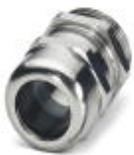
Cable gland, cable gland material: Nickel-plated brass, external cable diameter 15 mm ... 21 mm, shielding: no, connecting thread: M32 x 1.5, color: silver, with O-ring
