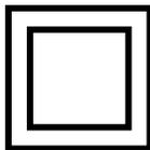
This equipment relies on double / reinforced insulation for safety and does not require a protective earth.
