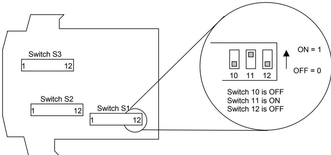
Switch S1 and S2 configure the input type and range, and switch S3 configures the output type, range and a few additional functions. The switch settings are explained in the next few pages. The diagrams refer to switch positions 0 and 1, with 0 being OFF and 1 being ON. This is illustrated in the picture above.
