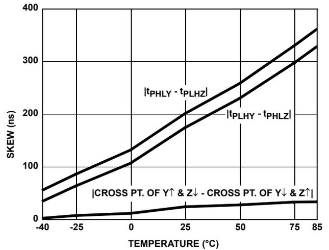
FIGURE 11. DRIVER SKEW vs TEMPERATURE (ISL8483, ISL8488, ISL8489)
