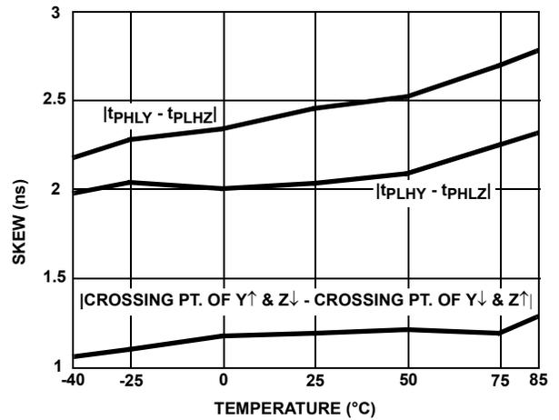
FIGURE 13. DRIVER SKEW vs TEMPERATURE (ISL8485, ISL8490, ISL8491)
