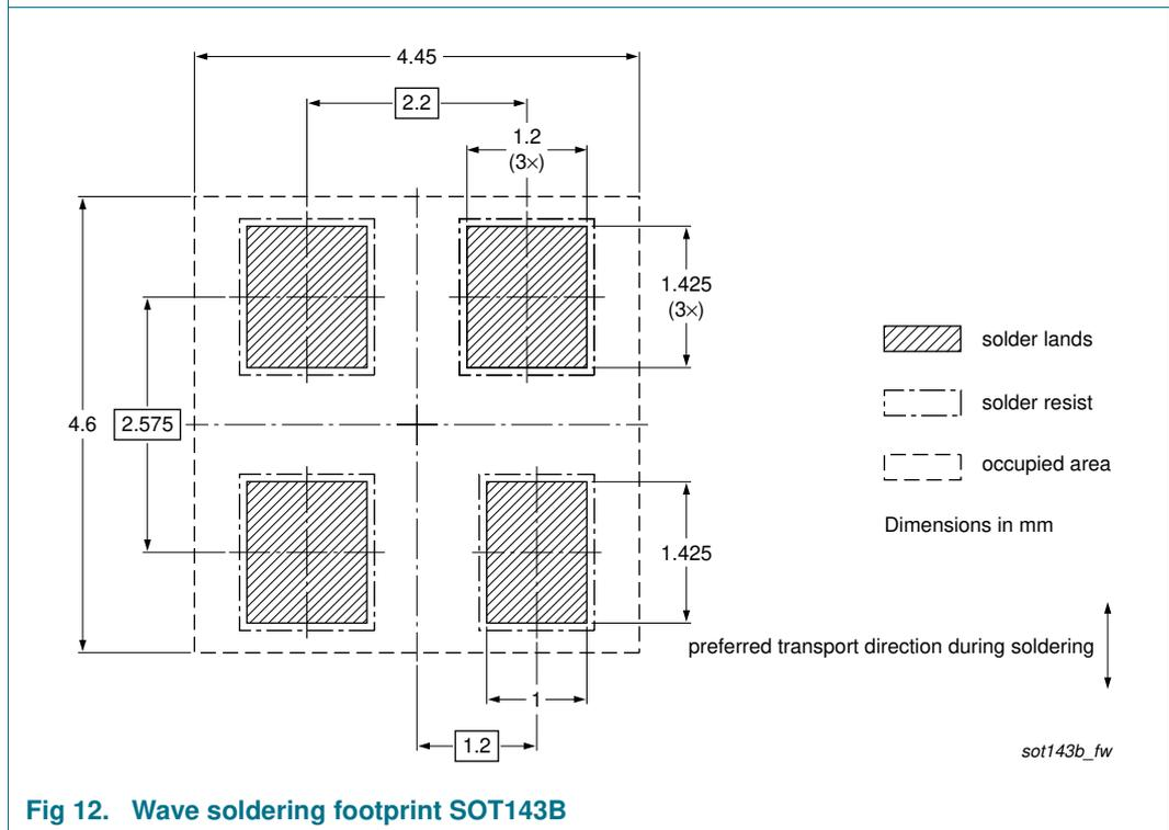
**Fig 12. Wave soldering footprint SOT143B**
