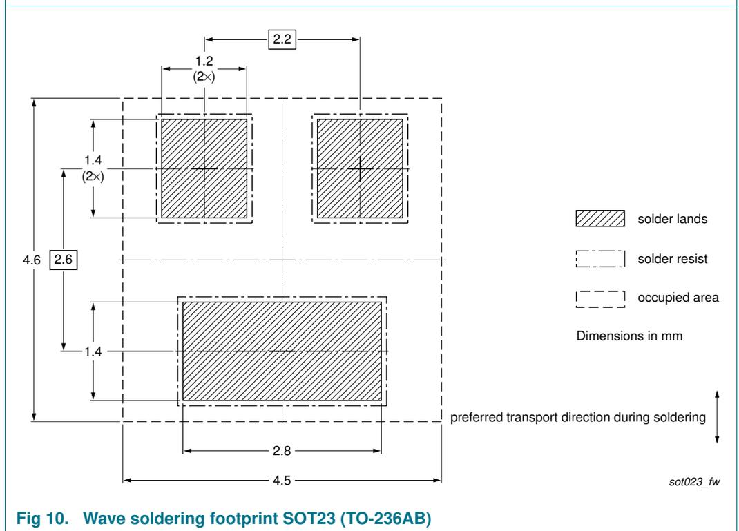
**Fig 10. Wave soldering footprint SOT23 (TO-236AB)**
