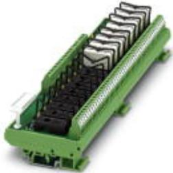
VARIOFACE module, for 16 plug-in miniature relays or miniature solid-state relays, with LED, negative switching, 24 V DC input voltage
