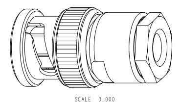
$-- \emptyset 12,70$ Ø9,53 — -STAMP "AMPHENOL 31-30220-1" —II.I HEX  $- \emptyset 14,50$ — 8,I3 — Ø3,10 Ø1,09 Ø 5,21 MUST CONFORM TO-AMPHENOL SPEC. 349-50551, SEC.301. -CONTACT -INSULATOR -CLAMP -NUT — 14.45 REF —— ---- 23.85 REF -
