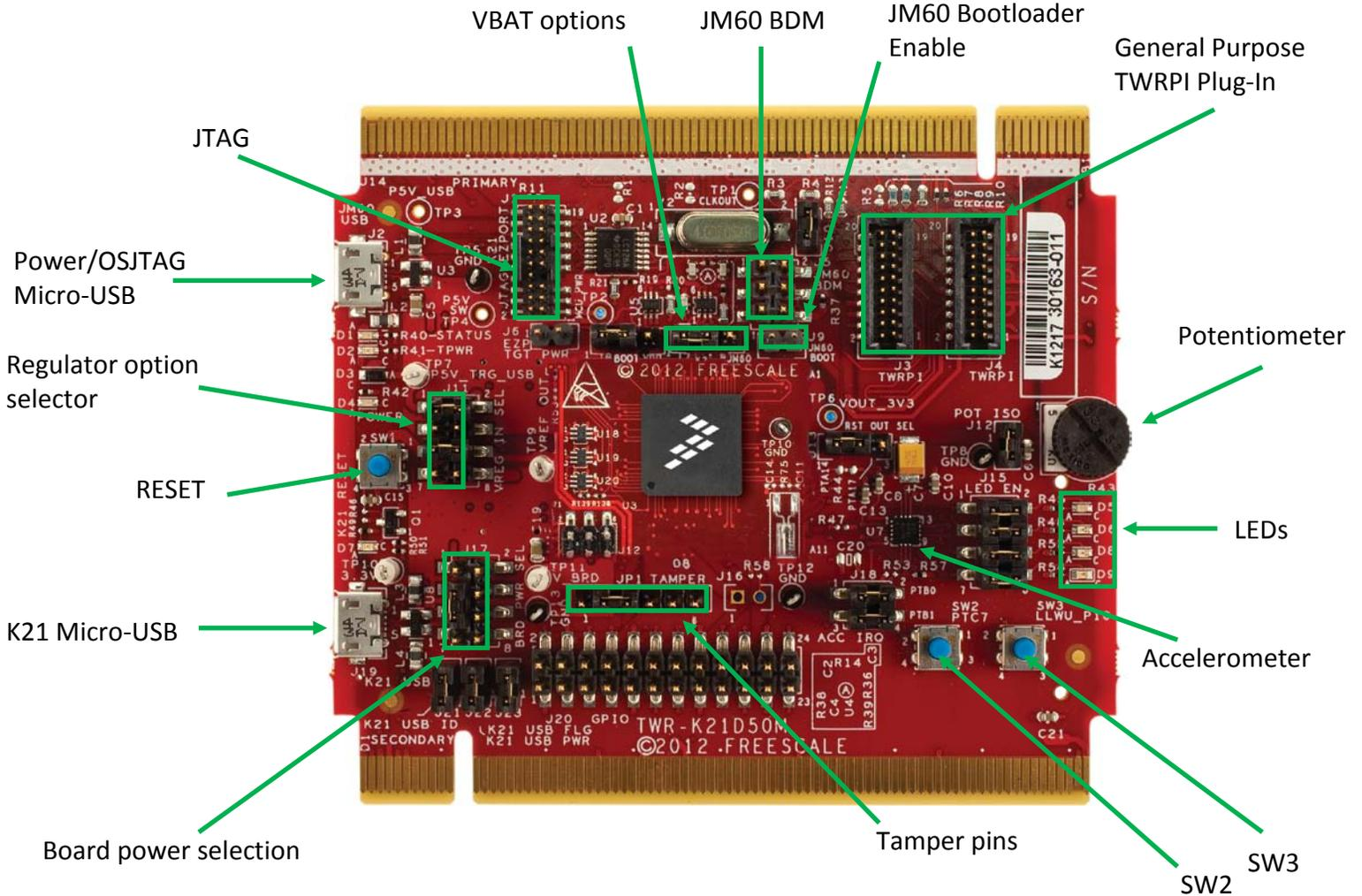
**Figure 2. Front side of TWR-K21D50M module
