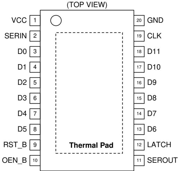
Figure 2. Pin Configuration
