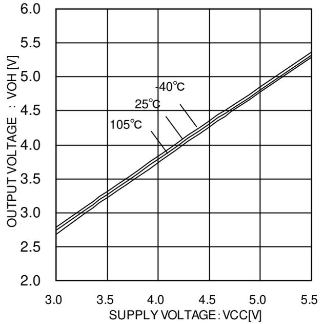
Figure 9. SEROUT high side voltage (VCC characteristic @ ISO=-4mA)
