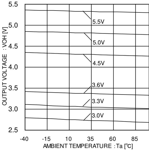
Figure 10. SEROUT high side voltage (Temperature characteristic @ ISO=-4mA)
