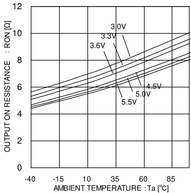
Figure 7. Output ON resistance (Temperature characteristic @ ID=20mA)
