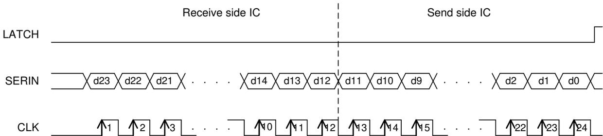
Figure 16. Cascade Connection
