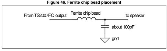
In the case where the distance between the TS2007FC output and the speaker terminals is too long, it is possible to have low frequency EMI issues due to the fact that the typical operating PWM frequency is 280 kHz and the fall and rise time of the output signal is less than or equal to 5 ns. In this configuration, it is necessary to use the output filter shown in *Figure 47*, that consists of L1, C1, L2, and C2 as close as possible to the TS2007FC outputs.
