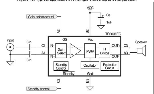
Figure 45. Typical application for single-ended input configuration
