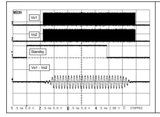
Figure 42. Startup and shutdown phase  $V_{CC}$  = 5 V, G = 6 dB,  $C_{in}$  = 1  $\mu F$ , inputs grounded
