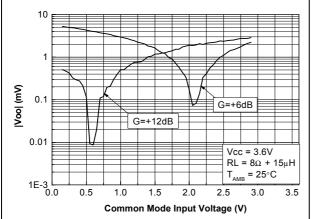
Figure 40. Output offset vs. common mode input voltage @ 2.7 V
