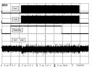
Figure 44. Startup and shutdown phase  $V_{CC}$  = 5 V, G = 12 dB,  $C_{in}$  = 1 µF,  $V_{in}$  = 1  $V_{pp}$ , F = 10 kHz
