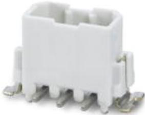
Header, Nominal current: 6 A, Rated voltage (III/2): 160 V, Number of positions: 6, Pitch: 2.5 mm, Color: white, Contact surface: Tin, Mounting: Taped SMD/THT/THR components
