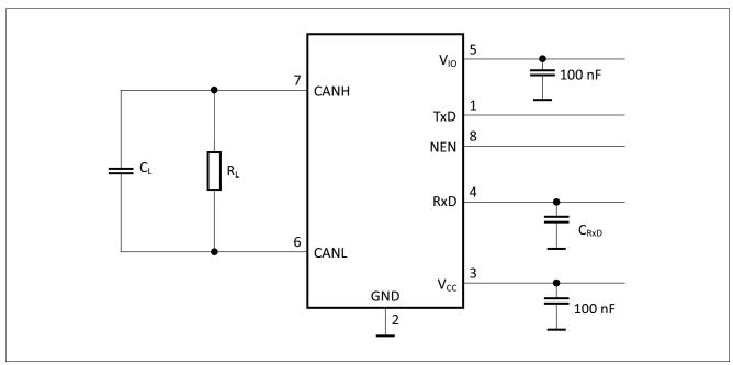
Figure 10 Test circuits for dynamic characteristics
