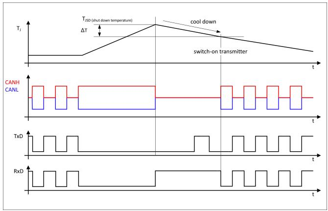
Figure 9 Overtemperature protection
