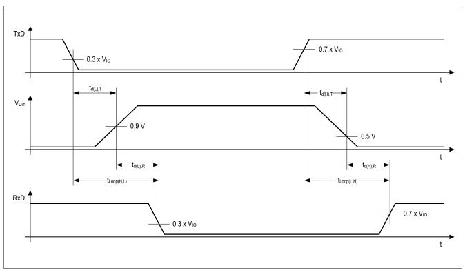
Figure 11 Timing diagrams for dynamic characteristics
