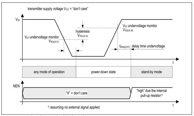
Figure 6 Undervoltage on the digital supply  $V_{10}$
