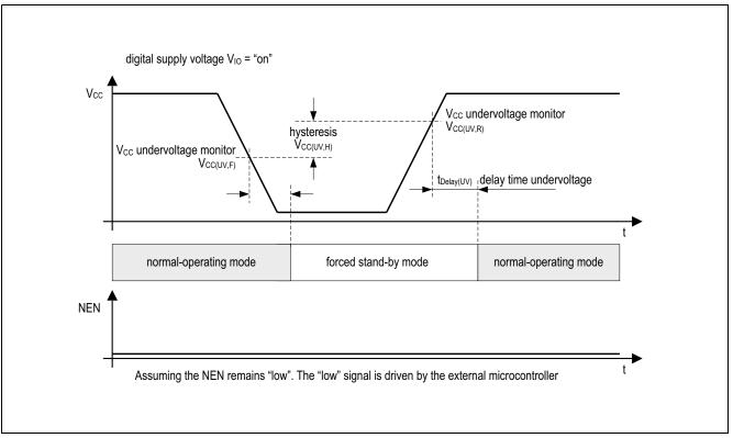
Figure 7 Undervoltage on the transmitter supply  $V_{cc}$
