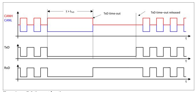
Figure 8 TxD time-out function
