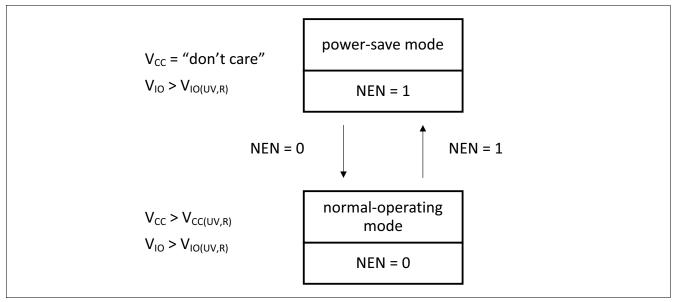
Figure 4 Mode state diagram
