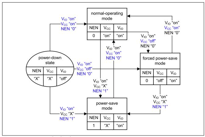
Figure 5 Power-up and undervoltage
