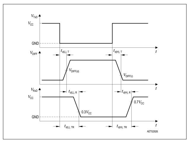
Figure 20 CAN Dynamic Characteristics Timing Diagram
