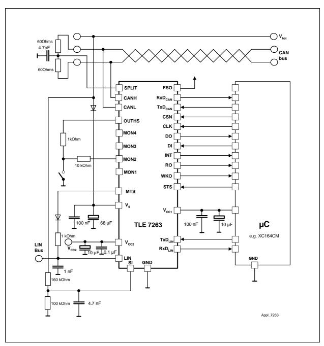
Figure 22 Application Circuit
