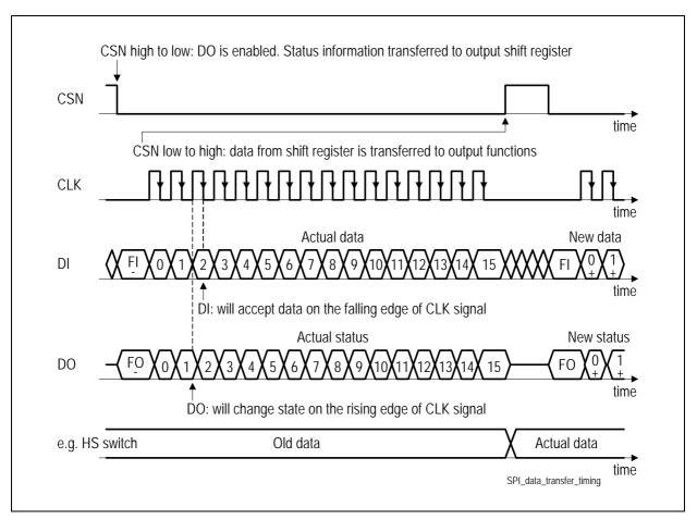
Figure 12 SPI-Data Transfer Timing
