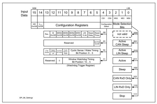
Figure 11 16-Bit SPI Input Data / Control Word
