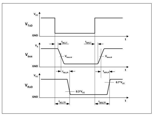
Figure 21 LIN Dynamic Characteristics Timing Diagram
