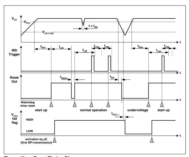
Figure 19 Reset Timing Diagram
