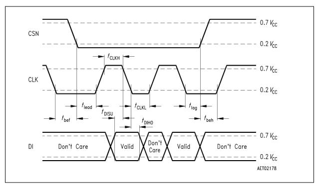
Figure 13 SPI-Input Timing
