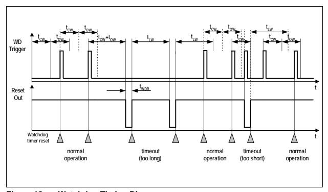
Figure 18 Watchdog Timing Diagram
