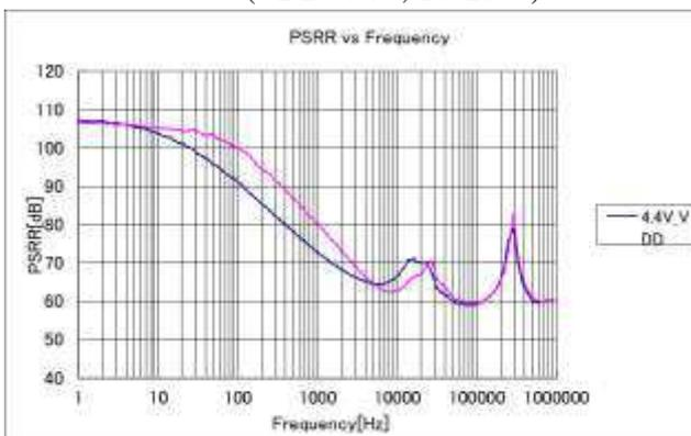
■ Power Supply Rejection Ratio vs. Frequency
