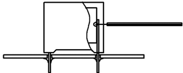
*Temperature monitored inside the capacitor.*
