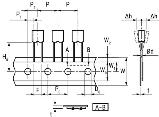
Figure 2 – Lead Spacing 7.5 mm
