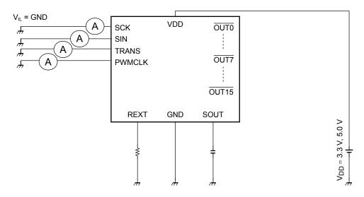
Test circuit 4: Power supply current
