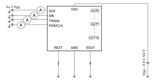
Test circuit 3: Low level logic input current
