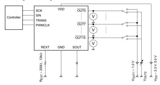
All output is set to turning on. Only one output is connected with the  $V_{OUT2}$  power supply, and other outputs are connected with the  $V_{OUT1}$  power supply.  $V_{OUT2}$  is changed and OOD voltage / OSD voltage is checked in the error detection result from each output terminal voltage and SOUT.
