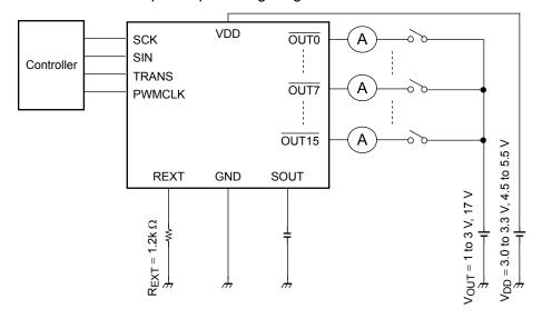
Test Circuit 6: OOD voltage / OSD voltage
