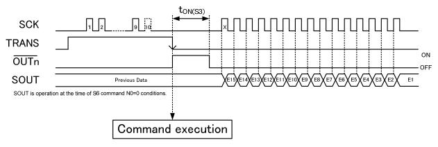
The first SCK (signal X) after this command is used for transmission of the output open/short detection result data. The input from SIN is not received. Note1
