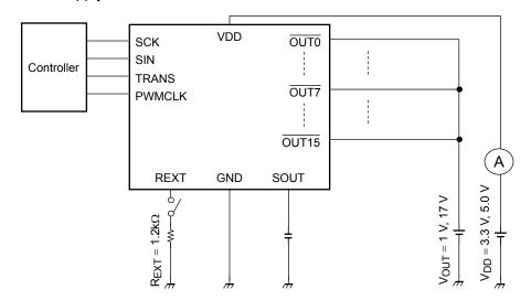
Test circuit 5 : Constant current error / Output OFF leak current
