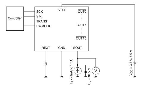
Test circuit 2: High level logic input current / Pull-down resistance
