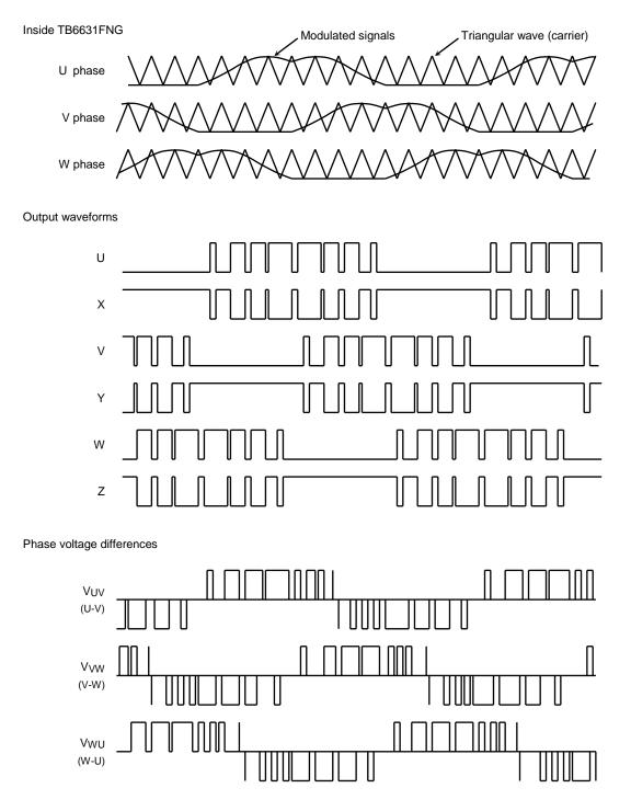
In sine-wave drive mode, the amplitude of the modulated signals varies with the VSP voltage, and the motor speed changes with the conduction duty cycle of the output waveforms. (See the sine-wave drive mode diagram on page 15.)
