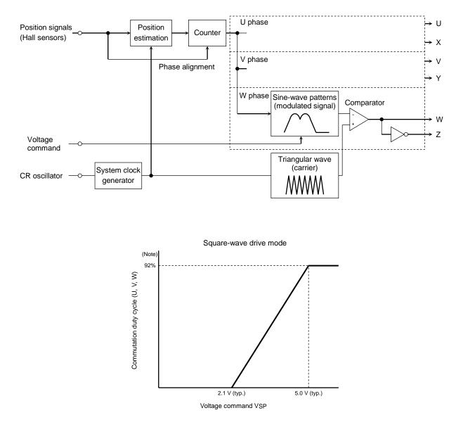
Note: The conduction period is reduced by the dead time. (carrier frequency  $\times$  92% – TD  $\times$  2)
