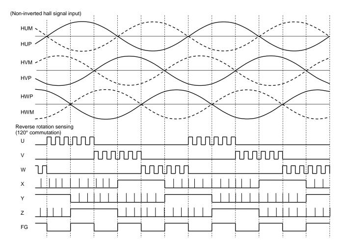
\*: When CW/CCW = High, non-inverted Hall signals put the TB6631FNG in 120° commutation mode with a lead angle of 0° (reverse rotation).
