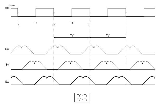
In the above diagram, the modulated waveforms have an interval  $(T_1)$  equal to the interval between a falling edge of HU to its next falling edge  $(T_1)$  of the previous cycle. If there is not an HU falling edge before  $T_1$  ends,  $T_2$  becomes equal to  $T_1$  until the next falling edge of HU.
