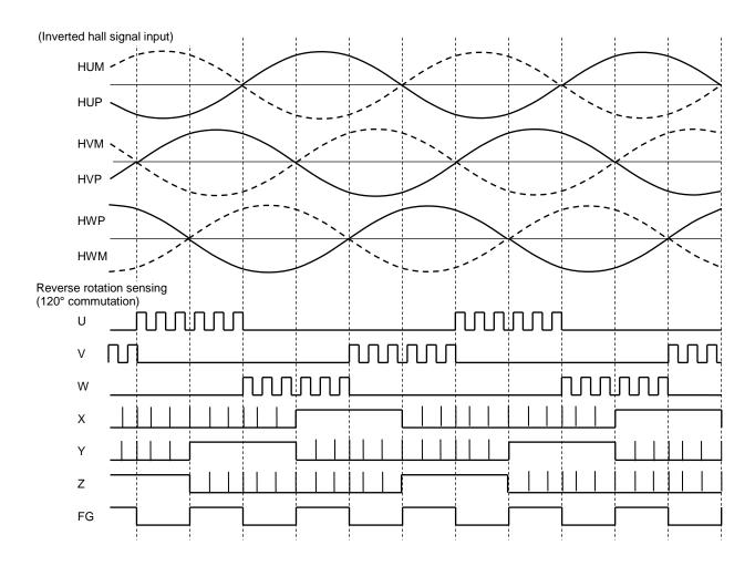
\*: When CW/CCW = Low, inverted Hall signals put the TB6631FNG in 120° commutation mode with a lead angle of 0° (reverse rotation).
