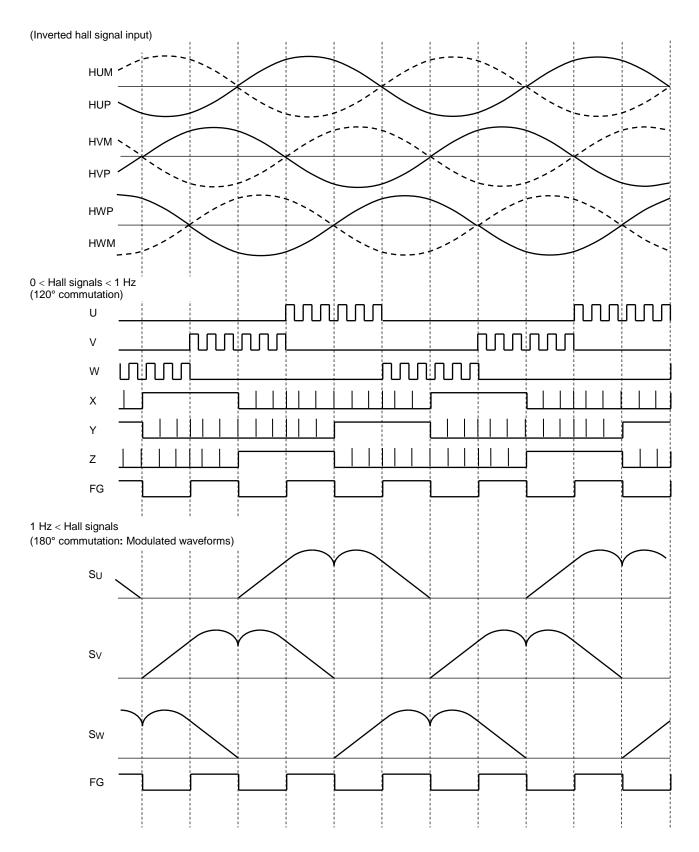
\*: When the Hall input frequency is equal to or greater than 1 Hz (@ fosc = 4 MHz), lead angle control is activated according the LA input.
