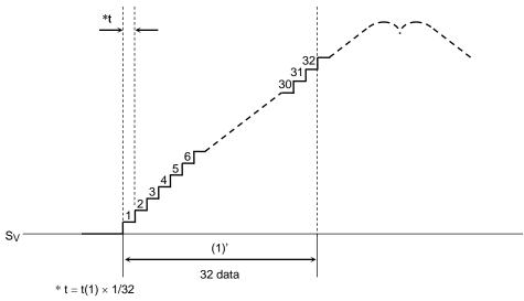
Phase of data and modulated waveform is adjusted for every zero cross of position detecting signal. Modulation is reset on each rising and falling edge of position detecting signal, which occurs every 60 electrical degrees. While the hall signal is out of its position and the motor is accelerating or decelerating, the modulated waveform becomes discontinuous upon each reset.
