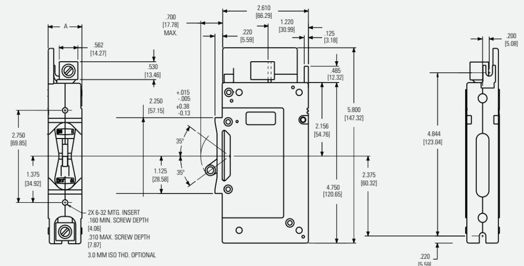
Back Connected Stud Terminal (Front Mounted)
