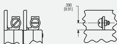
Slotted Mounting Bracket terminal codes -2, -3, -5, -7, -3M, -5M, -7M
