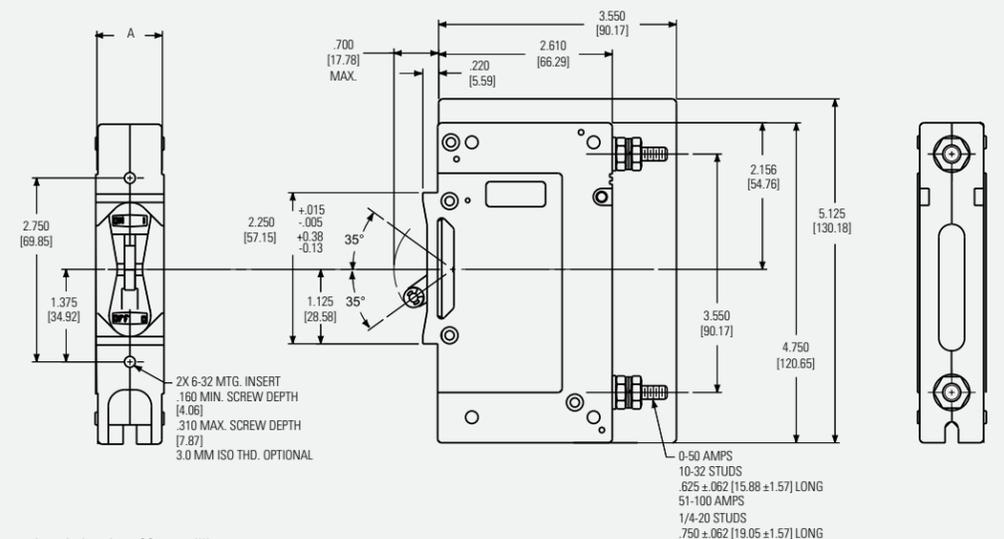
Note: Tolerance ± .015 [.38] unless noted. Dimensions in brackets [ ] are millimeters.
