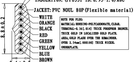
$2.4 \pm 0.2$ SEC: A=A NOTE FOR PLUG: MATERIAL: HOUSING-POLYCARBONATE, CLEAR. TERMINAL-0. 36 [. 014] THICK PHOSPHOR BRONZE. THICK GOLD IN LOCALIZED GOLD PLATE. AREA, GOLD FLASH OVER THE REMAINDER. OVER 2.54um[.000100] THICK NICKEL UNDERPLATE.
