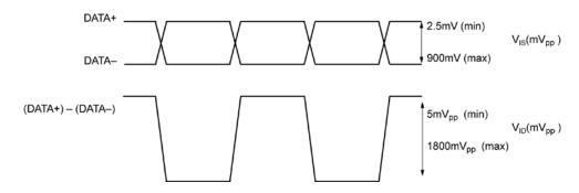
Figure 1.  $V_{\text{IS}}$  and  $V_{\text{ID}}$  Definition
