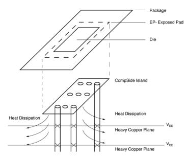
PCB Thermal Consideration for 16-Pin QFN Package
