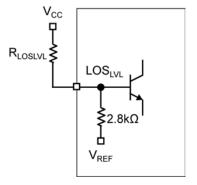
Figure 5. LOS<sub>LVL</sub> Setting Circuit
