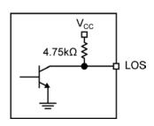
Figure 4. Input Structure
