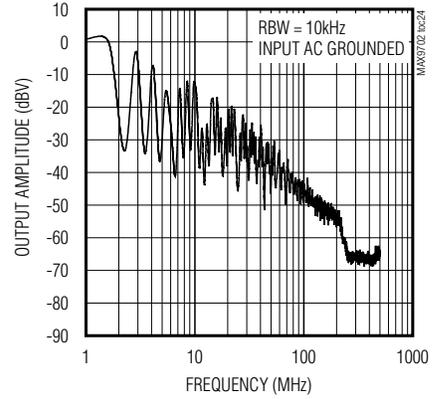
**WIDEBAND OUTPUT SPECTRUM (SSM MODE, SPEAKER MODE)**
