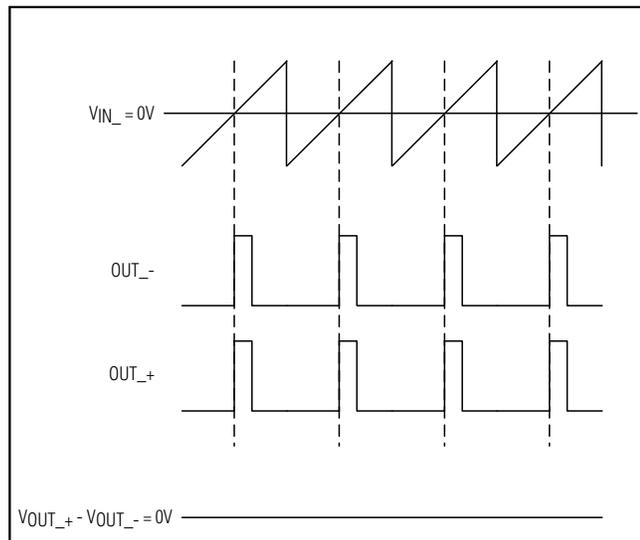
Figure 5. MAX9702 Outputs with No Input Signal
