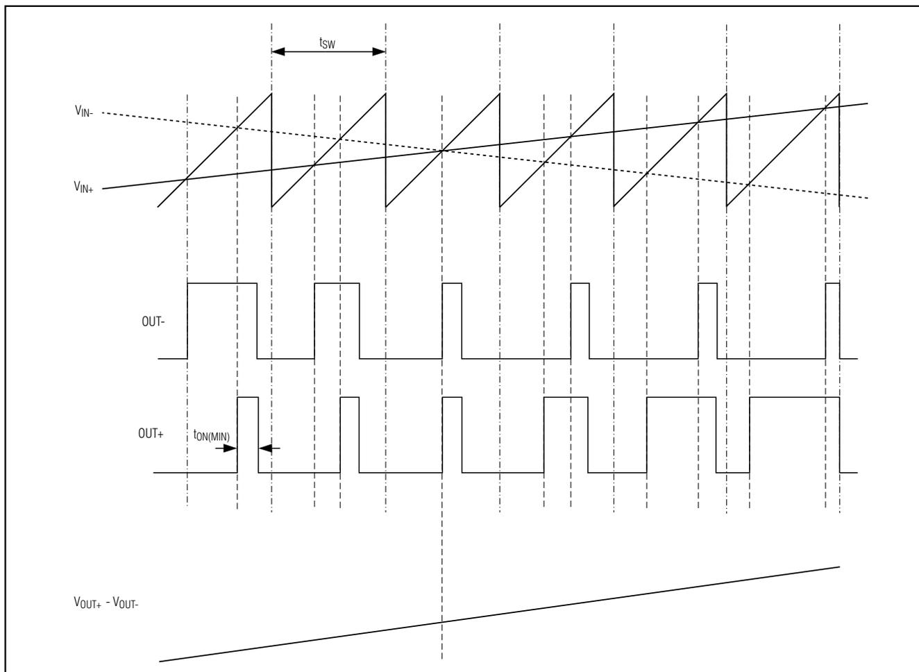
Figure 1. MAX9702 Outputs with an Input Signal Applied
