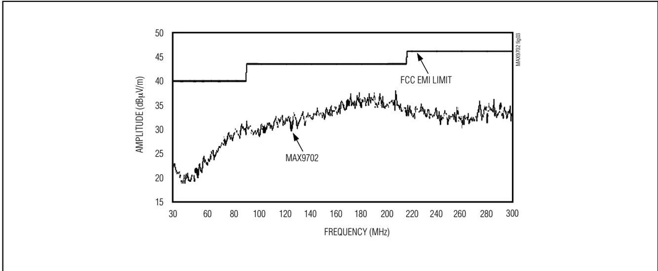
Figure 3. MAX9702 EMI with 76mm of Speaker Cable
