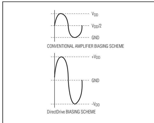
Figure 7. Traditional Amplifier Output vs. MAX9702 DirectDrive Output
