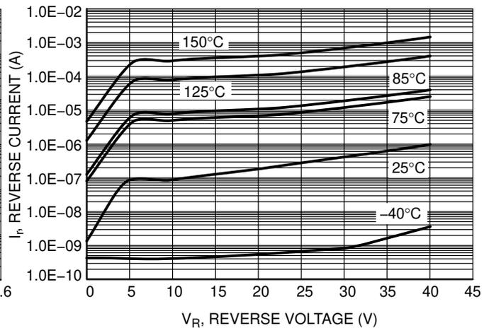
Figure 2. Leakage Current
