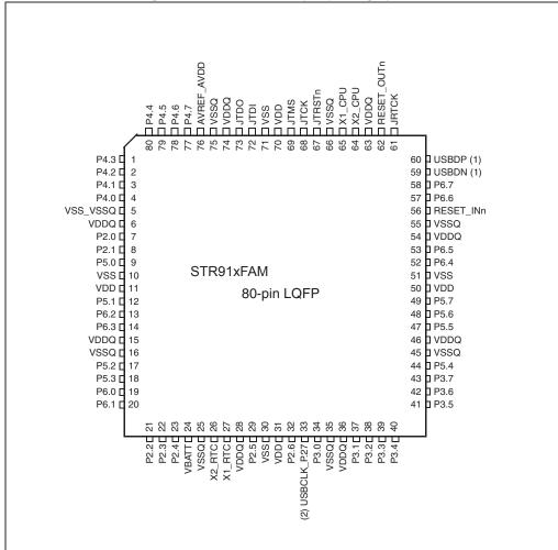
Figure 7. STR91xFAM 80-pin package pinout
