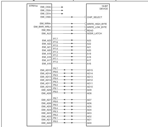
Figure 4. EMI 16-bit multiplexed connection example
