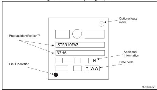
Figure 46. LFBGA144 package top view
