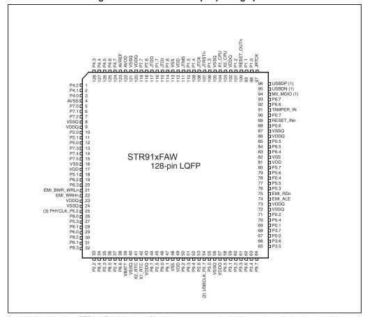
Figure 8. STR91xFAW 128-pin package pinout
