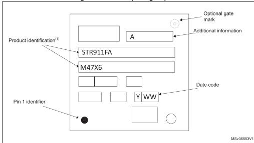
Figure 42. LQFP80 package top view
