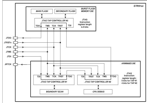
Figure 3. JTAG chaining inside the STR91xFA
