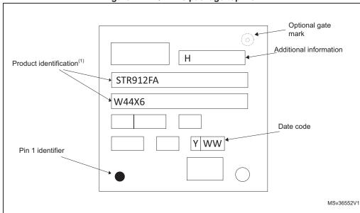
Figure 44. LQFP128 package top view
