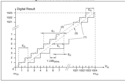
Figure 33. ADC conversion characteristics
