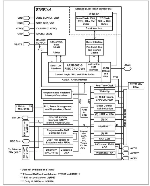
Figure 1. STR91xFA block diagram
