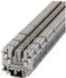
Basic termination blocks with test connection on both sides and double connections with the same potential for NS 32 and NS 35/7.5 DIN rail, with end cover, for ST-REL..., ST-OV... and ST-OE... plugs, 3-pos.
