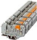
Basic termination blocks with test connection on both sides and knife disconnection for NS 32 and NS 35/7.5 DIN rail, with end cover, for ST-REL..., ST-OV... and ST-OE... plugs, 3-pos.
