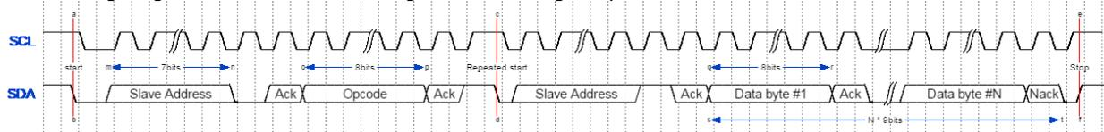
**Figure 8: Read message transfer using a repeated start (I<sup>2</sup>C)**
