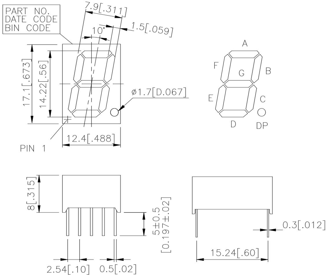
NOTES: All dimensions are in millimeters. Tolerance is  $\pm 0.25$ -mm (0.01") unless otherwise noted.
