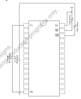
In system power mode, both V $_{CC}$  and V $_{CAP}$  are connected to the +5V power supply without the 68  $\mu F$  capacitor. In this mode, the AutoStore function of the STK12C68 operates on the stored system charge as power goes down. The user must, however, guarantee that V $_{CC}$  does not drop below 3.6V during the 10 ms STORE cycle.
