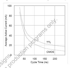
Figure 5. Current Versus Cycle Time (Write)
