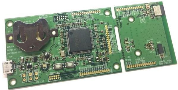
The MBN52832 Development Kit is designed to facilitate application development using the Nordic nRF52 SDK. The EVB supports the same J-Link USB-SWD and USB-UART interfaces as those provided by the nRF52 DK to ease the debugging and development process.
