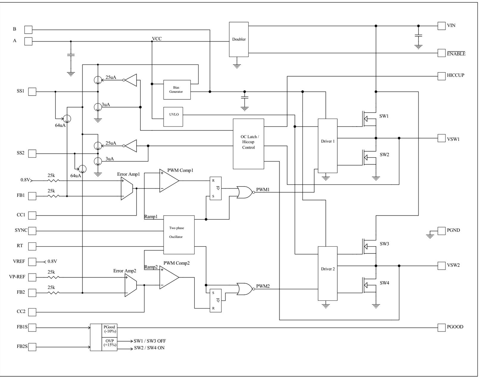
Fig. 1: IP1201PbF Internal Block Diagram
