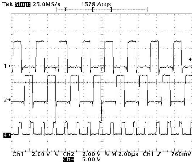
Ch1: Output 1 switching node, 400kHz
