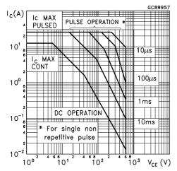
Figure 4: Derating Curve
