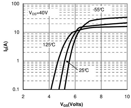
**Figure 2: Transfer Characteristics**
