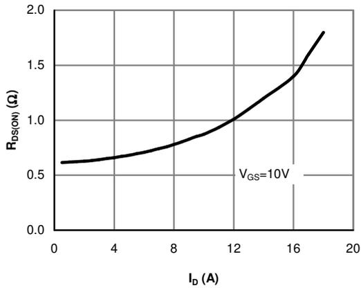
**Figure 3: On-Resistance vs. Drain Current and Gate Voltage**
