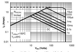
Figure 9: Maximum Forward Biased Safe Operating Area for AOT9N50 (Note F)
