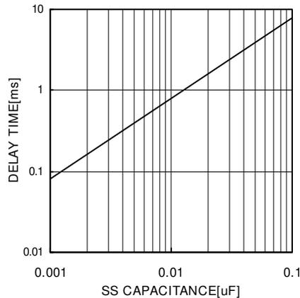
Fig. 34 SS Pin Capacitance vs Delay Time
