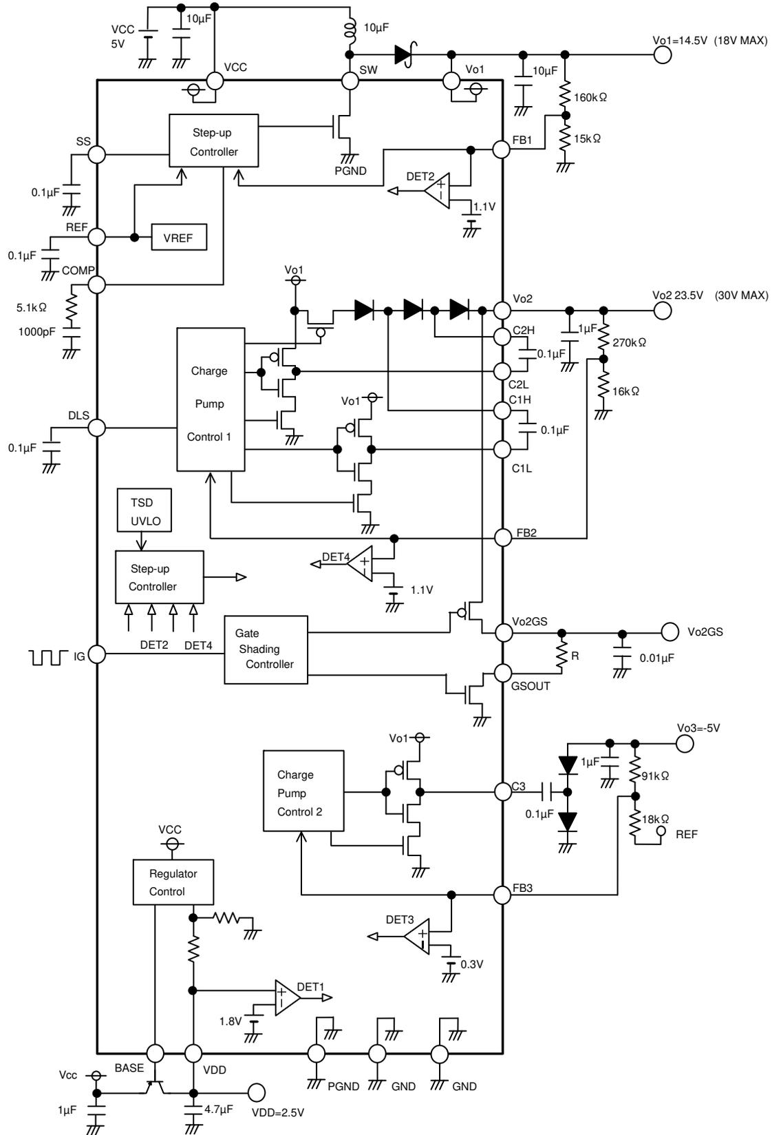
Fig. 25 Block Diagram
