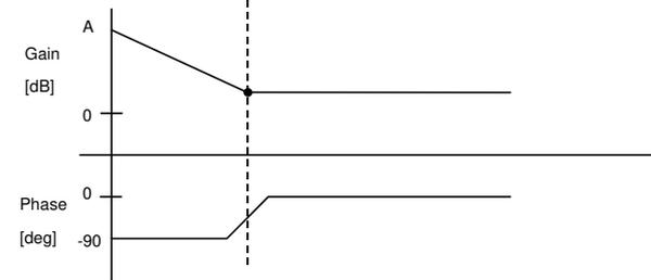
$$F_p = \frac{1}{2 \pi \times R_o \times C_o} \text{ [Hz]}$$
