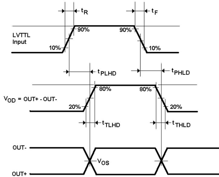
FIGURE 4. LVTTTL Input to LVDS Output AC Waveform
