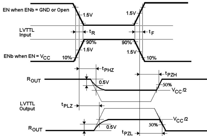
FIGURE 10. LVTTTL Output Enable / Disable Timing Waveforms
