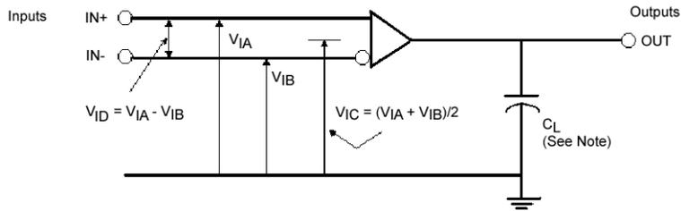
Note:  $C_L = 15\text{pF}$ , includes all probe and jig capacitances
