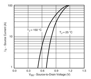
**Source Drain Diode Forward Voltage**
