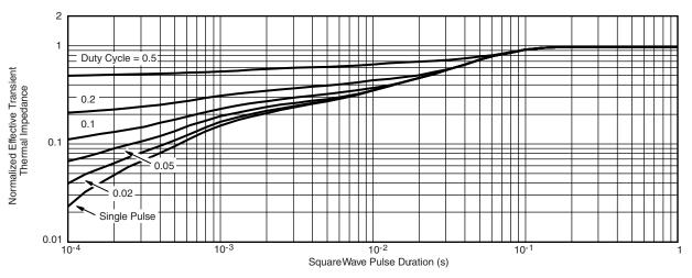
Normalized Thermal Transient Impedance, Junction-to-Case
