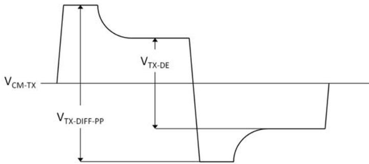
Figure 9. Transmitter Differential Voltage
