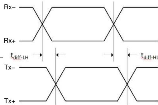
Figure 10. Propagation Delay
