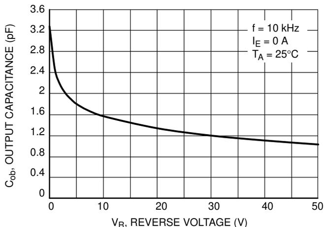
Figure 4. Output Capacitance
