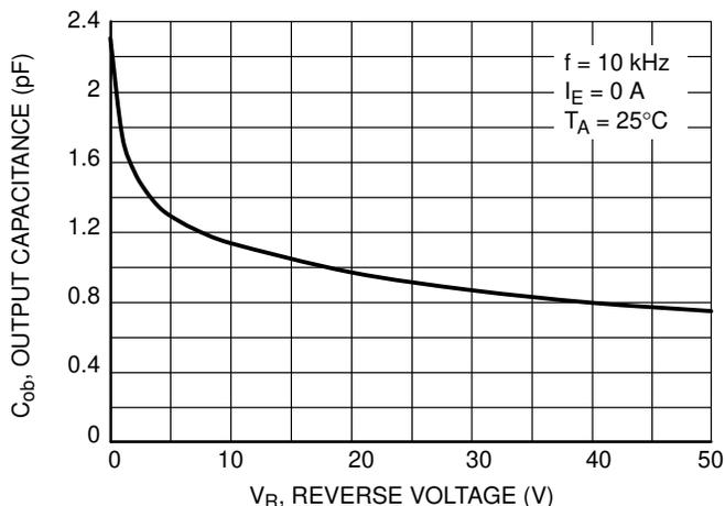
Figure 9. Output Capacitance
