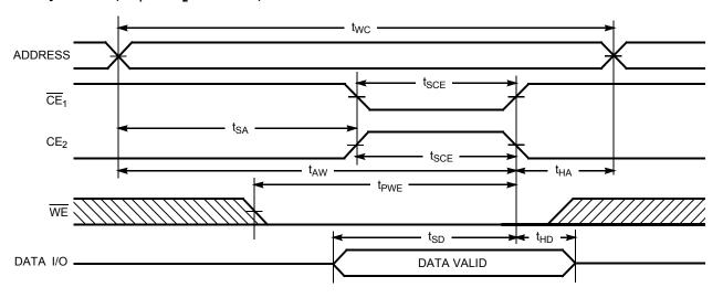
14. Address valid prior to or coincident with  $\overline{CE}_1$  transition LOW and  $CE_2$  transition HIGH.
