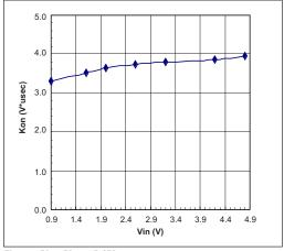
$K_{ON}$  vs.  $V_{IN}$ ,  $V_{OUT}$ =5.0V
