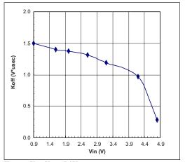
$\overline{K_{OFF}}$  vs.  $V_{IN}$ ,  $V_{OUT}$ =5.0V
