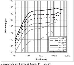
Efficiency vs. Current Load, V<sub>OUT</sub>=5.0V
