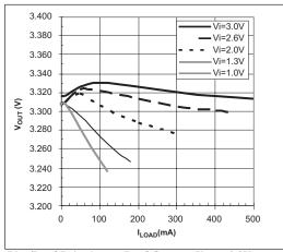
Line/Load Rejection vs. Load Current,  $V_{OUT} = 3.3V$
