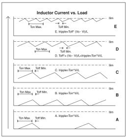
Figure 1. Inductor Current vs. Load
