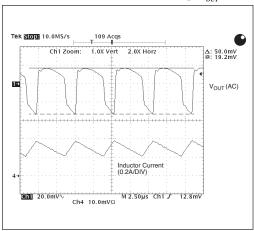
Output Ripple,  $V_{IN}$ =2.6V,  $I_{LOAD}$ =200mA,  $V_{OUT}$ =3.3V
