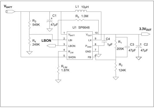
SP6648EB Evaluation Board Schematic
