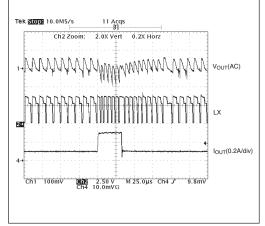
Load Step, 0.1A to 0.3A,  $V_{IN} = 2.6V$ ,  $V_{OUT} = 3.3V$
