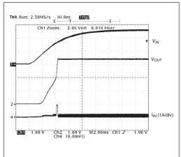
Startup,  $V_{IN}$ =2.6V,  $V_{OUT}$ =3.3V,  $R_{LOAD}$  = 100 $\Omega$
