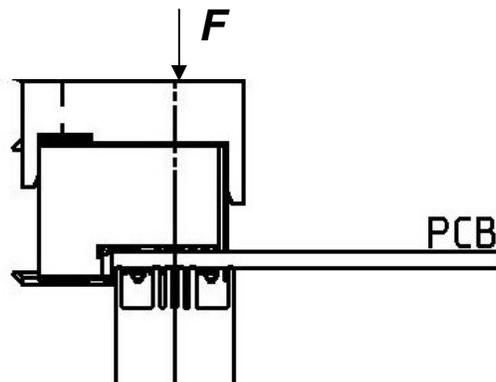
Figure 12 – Applying Force
