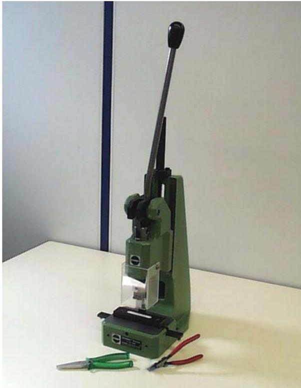
**Figure 17 -- Connector Removal tooling HM2Y350**
