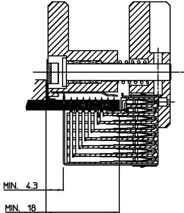
**Figure 15 - Clip on Cover Shield Tool HM2Y290**
