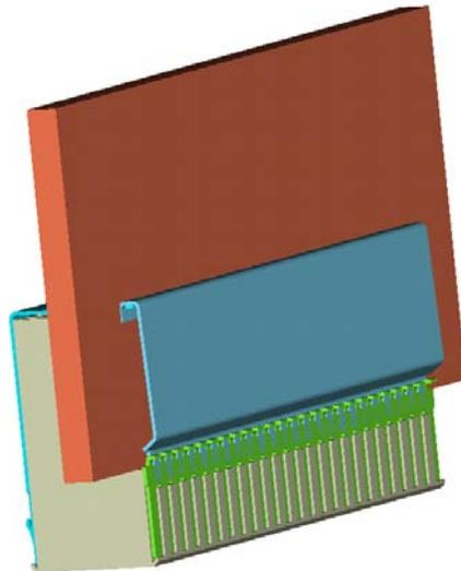
**Figure 13 – Clip on cover shield**
