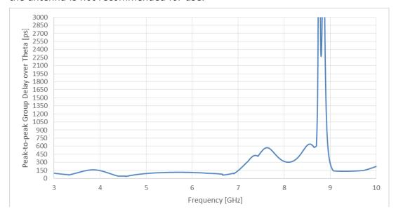
The measured Group Delay variation for the FXUBW10 antenna is presented in the graph above. This translates into maximum distance error introduced by antenna as presented below.
