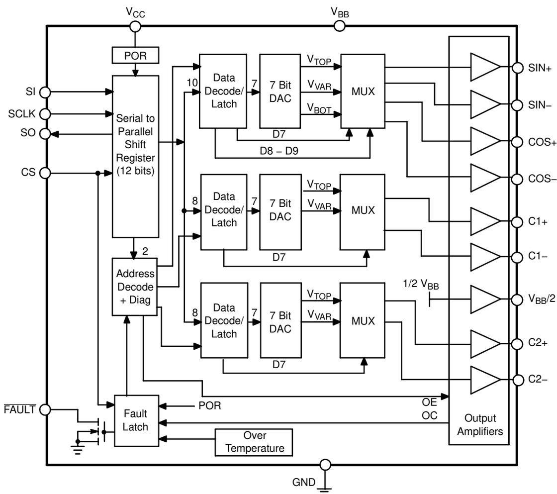
Figure 1. Block Diagram
