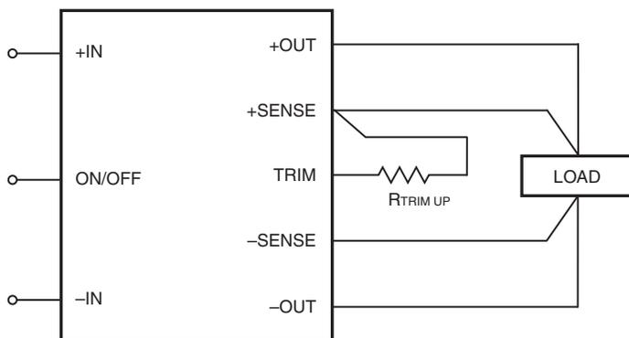
Figure 6. Trim Connections to Increase Output Voltages
