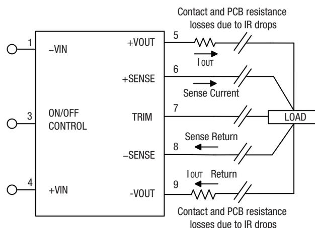
Figure 4. Remote Sense Circuit Configuration
