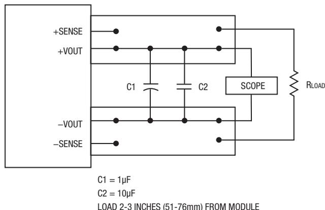
**Figure 3. Measuring Output Ripple and Noise (PARD)**
