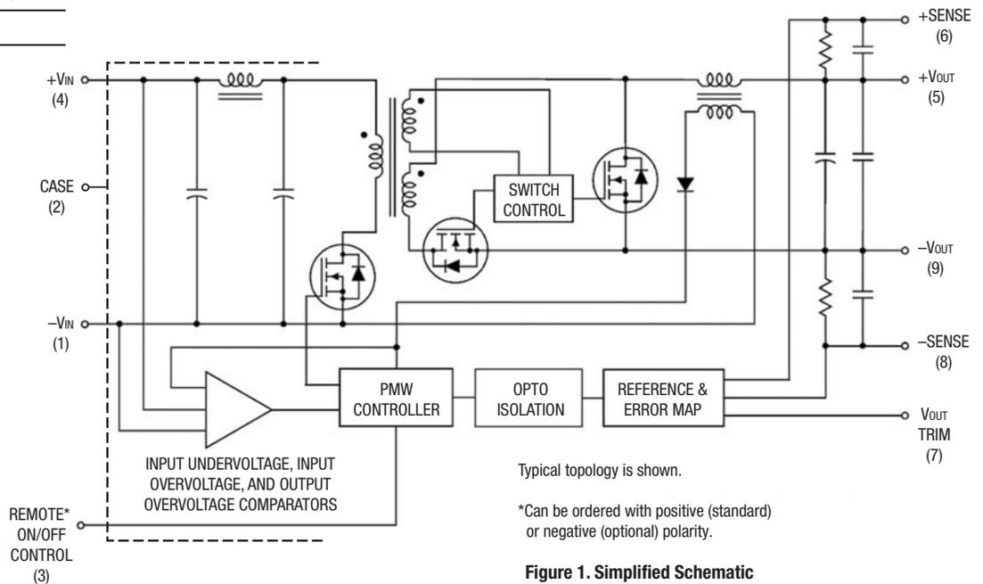
Figure 1. Simplified Schematic
