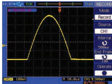
Monitor and analyze long term signal behavior by recording data continuously over an extensive period of time and playing it back for post acquisition analysis. Data is recorded in a sequence of up to 1000 frames of 4 k data points each and the time interval between each frame is adjustable from 1 ms – 100 s. The data can be saved in a single file to internal memory or USB flash drive.
