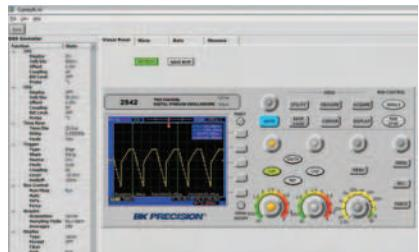
The included Comsoft PC software provides full access to the oscilloscope's display, measurements waveform data and front panel controls through the rear panel USB device port.
