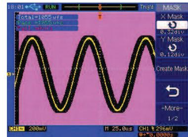
Create a user defined mask (pass/fail limits) and automatically compare it against the input signal from CH1 or CH2. This feature is ideal for manufacturing test applications that require instant go/no go test results.
