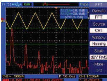
Display and measure the input signal's frequency spectrum. Select one of the 5 FFT windows: Rectangular, Hanning, Hamming, Blackman and Flatop. Use cursors to measure the spectral component's magnitude and frequency.
